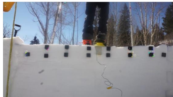
Figure 2. PTV software particle prioritization and tracking procedure. A screen capture from the live particle tracking process to illustrate particle corner prioritization and associated number scheme.
