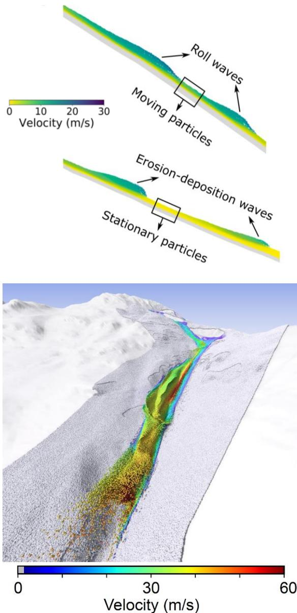
Figure 6: MPM simulations of snow avalanches over an erodible bed in a) 2D showing the natural emergence of rollwaves and erosion deposition waves and b) 3D on complex topography for the 2019 Salezer avalanche (Kyburz et al., 2023).
