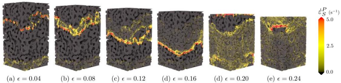
Figure 1: Snapshots of the plastic shear strain rate in a three-dimensional microstructure-based MPM simulation (Blatny et al. 2023).
