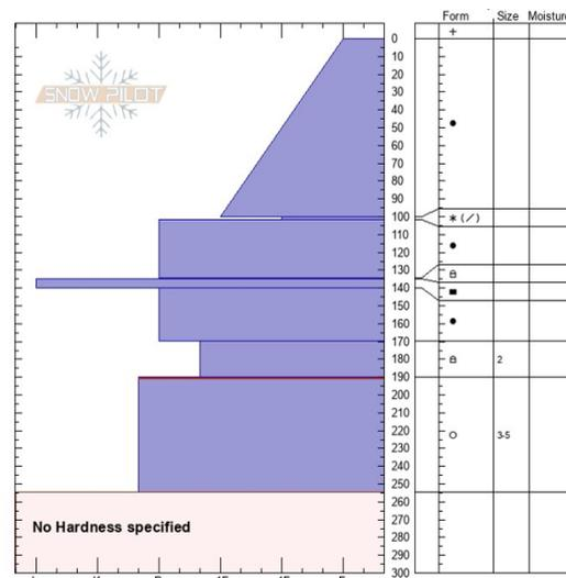
Figure 4: Crown Profile of the Jan 29 avalanche in Alyeska's Christmas Chute. The avalanche failed on the 1F+ hard layer of rounding facets at 170-190 cm. Halloween crust is 190-250 cm, and New Year's crust is 135-140 cm.
