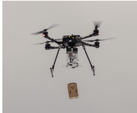
Image 1 – Drone Amplified modified Alta X dropping inert payload out of Maple Leaf Products modified Sentinel 6000 Prototype during testing February 2023.
