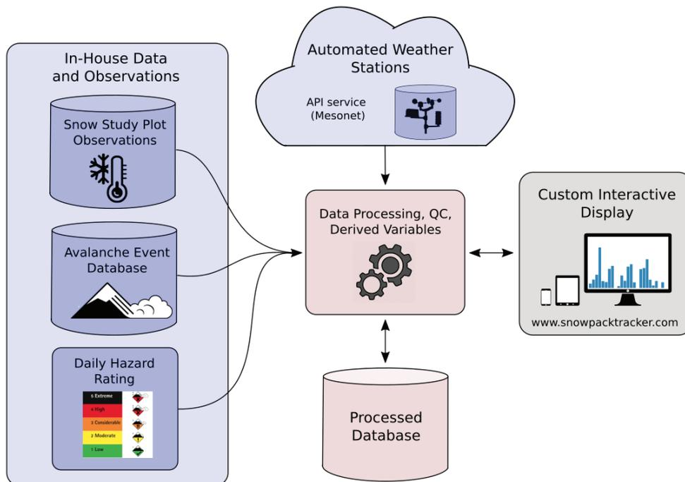
Figure 5. Schematic showing the general flow of data ingest, data processing, and rendering of the web display.
