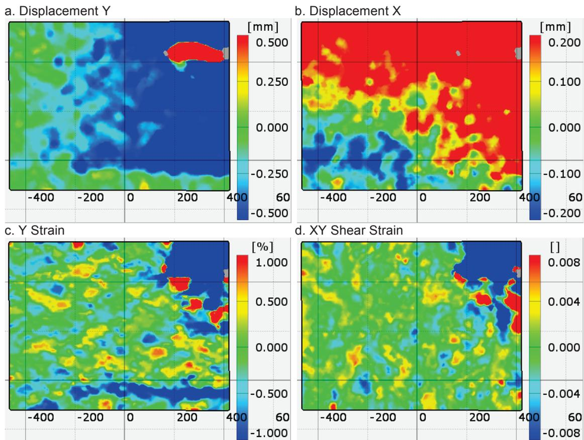
Figure 5: Particle tracking data of the A1 ECTP during propagation. In this example, the horizontal displacement along the weak layer is less significant than in other tests, and the shear strain is hard to pick out. Positive X direction is to the right and positive Y direction is up.
