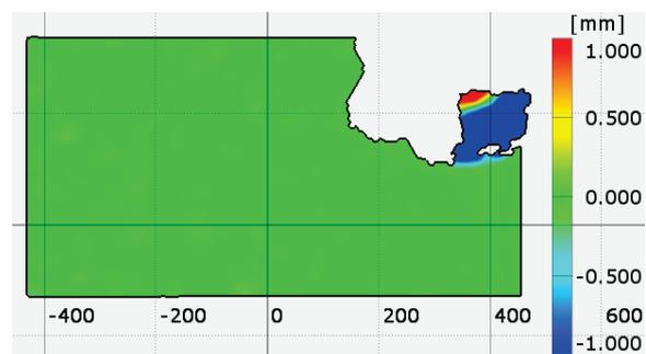
Figure 2: Particle tracking displacement Y data of E1 ECTP just before crack initiation and propagation. Positive X direction is to the right and positive Y direction is up.
