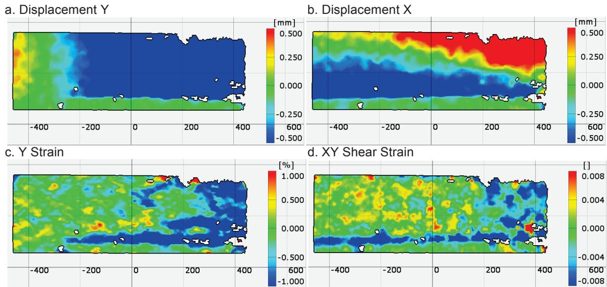
Figure 4: Particle tracking data of the F1 ECTP just after the shear strain reaches the far end of the column. In this example, the shear strain reaches the far end of the column before the collapse does. Positive X direction is to the right and positive Y direction is up.
