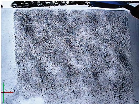
Figure 1: A picture of the E1 ECT after the dot pattern was sprayed onto the face of the column, but before any tapping occurred.
