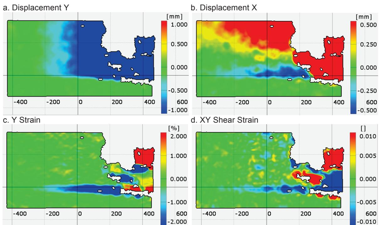
Figure 3: Particle tracking data of the E1 ECTP during crack propagation. Positive X direction is to the right and positive Y direction is up.
