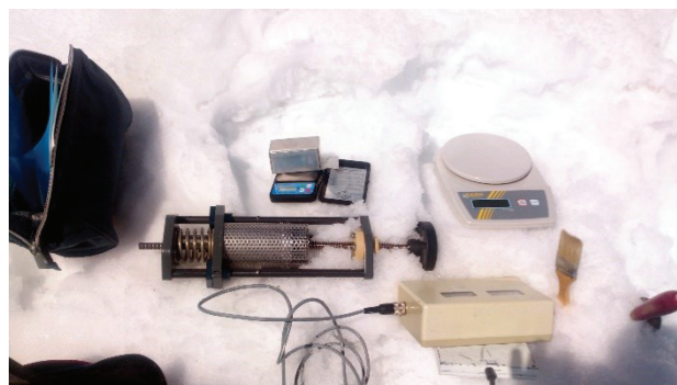
Figure 3: Foto of equipment in the field: electronic scale, aluminium quadrat for measuring snow density, Denoth meter, brush, SNOWPRESS (photo by R. Fromm, 18 April 2018).
