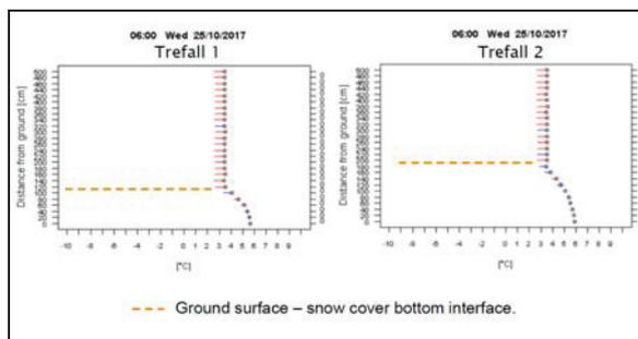
Figure 3: Temperature sensors showing temperature the day after installation. Temperature in the ground increases with depth. Both Trefall 1 and Trefall 2 showed the same temperature (ca 5.5°C) at 120 cm depth.
