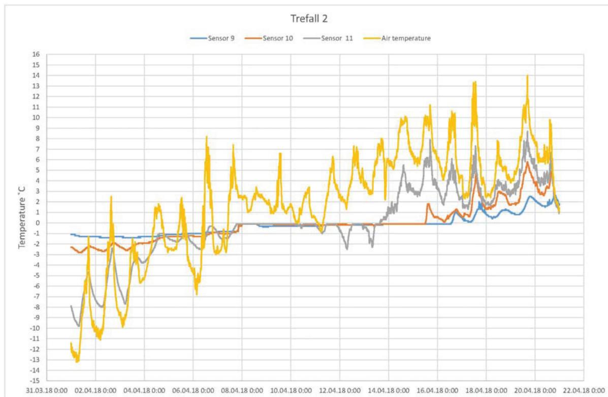
Figure 14: Air temperature, the sensor closest in the snow closest to the ground – sensor 11, sensor 10 – the upper most sensor in the ground and sensor 9 - 20 cm further down.
