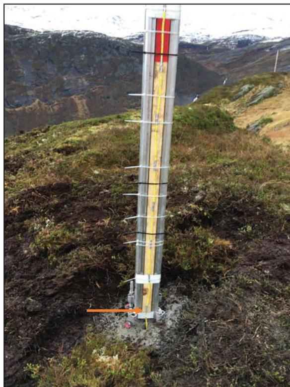
Figure 2: The temperature sensors are placed every 20 cm. The orange arrow points at the temperature sensor closest to the ground surface. The next temperature sensor below is placed beneath the ground surface. Picture is from Trefall 1.
