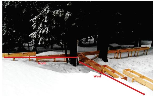
Figure 2: Snow interception measurement device.
