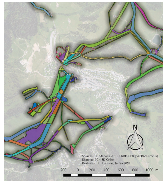
Figure 2: Example of the discretization of a ski resort into SRUs based on the topographic characteristics of the slopes and the presence/absence of snow guns.
