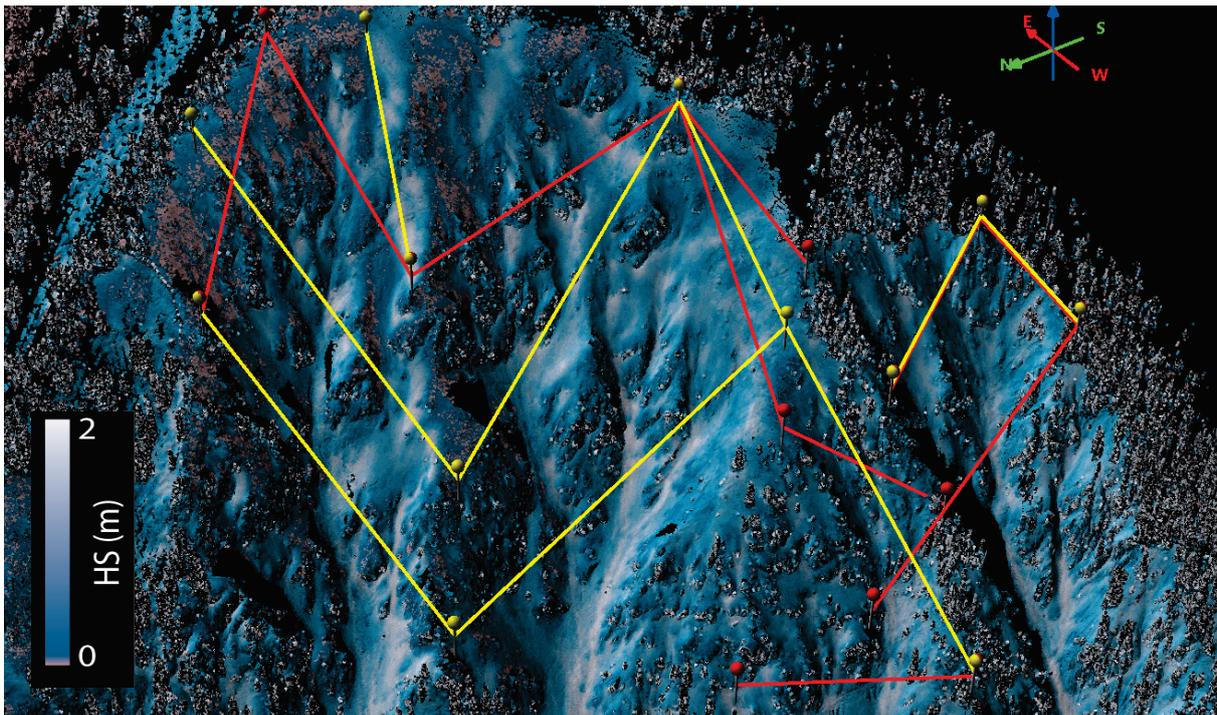
Figure 2: Initial (red) and re-designed (yellow) explosive tramway network for the Steep Gullies expansion area at A-Basin, overlaid on a TLS snow depth map (from Deems et al., 2016).
