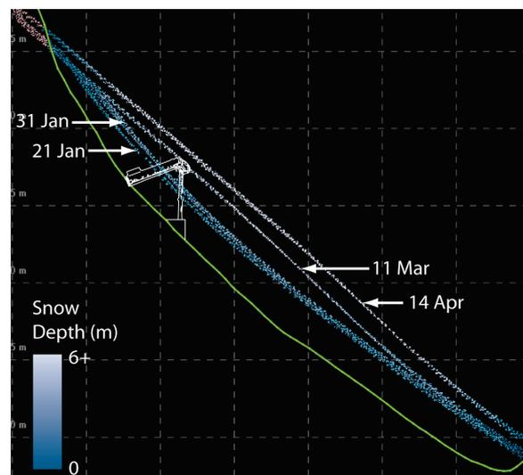
Figure 3: Time series cross-section of snow depth through the 1Low Gazex exploder, Loveland Pass, CO.
