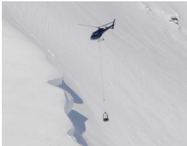
Fig. 4: Active avalanche control with Daisybell, here used near the city of Tromsø, Northern Norway. (Photo: Ole-André Helgaas)
