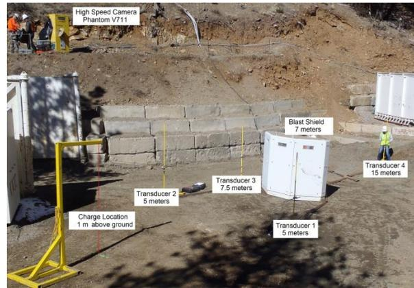
Fig. 7: Experimental setup test series B.
