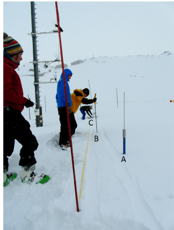
Fig. 1: Transect with side-by-side hardness measurements with the ramsonde (A) the SP2 (B) and the SMP (C) at the Weissfluhjoch study plot.
