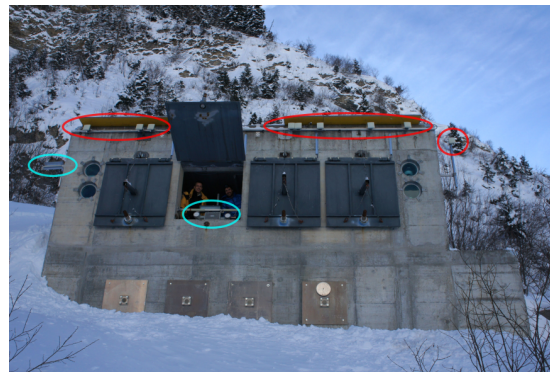
Figure 1: Set up at the Vallée de la Sionne test site with Doppler and GEODAR antennas on the outside of the bunker (l.t.r. Jim McElwaine, Anselm Köhler).
