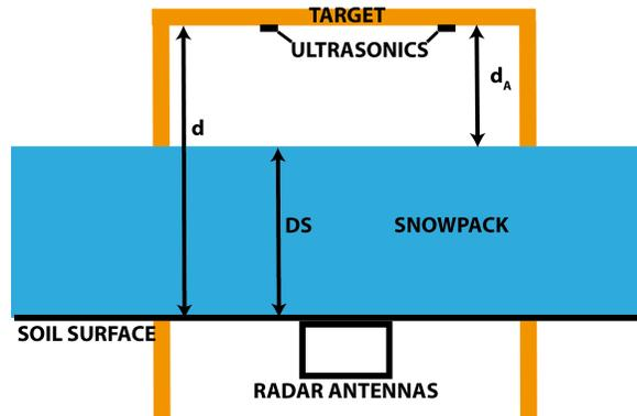
Fig. 2: Sketch showing the setup for the upGPR measurements at the Dorfberg site. The wooden construction holding the ultrasonic sensors is displayed in orange.
