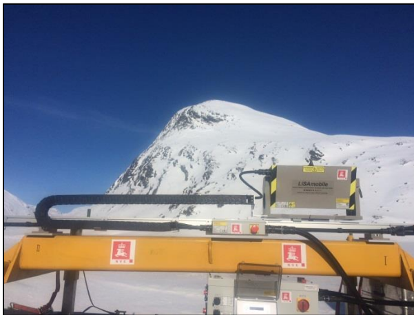
Fig. 2: The radar on a movable fundament, measuring at Stavbrekka.
