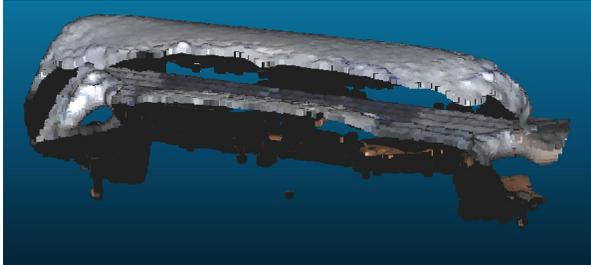
Fig 4. Looking from the side at the roof of the building with both models present. The top layer is the snow from the winter model and the bottom layer is the roof of the building from the spring model.
