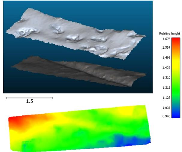
Fig 5. A patch of snow in front of the building. The top layer is the snow with footsteps present and the bottom layer is the snow-free ground surface with a drainage ditch. The relative height is in metres and is looking down on the snow surface.
