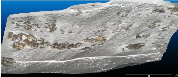
Fig 6. Avalanche starting zone and crown modelled using five photographs.
