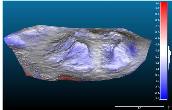
Fig 2. Change detection for quinzee study site, with the spring model shown. Differences are measured in metres, with blue showing snow loss and red showing snow gain.
