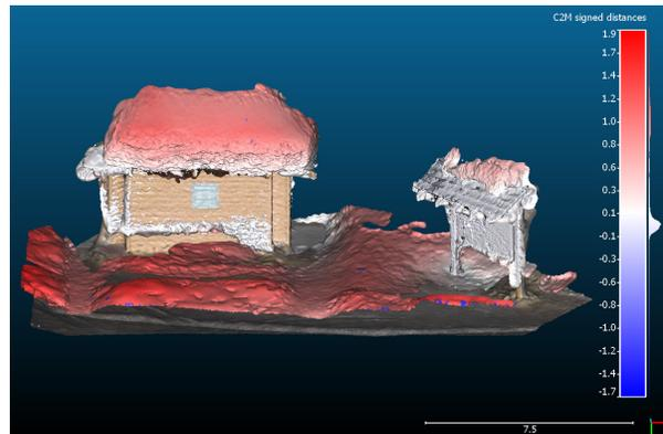
Fig 3. Change detection for the building study site. Both models are shown, with the change detection colours on the winter model and real-life colours shown for the spring model. Differences are measured in metres, with blue indicating snow loss and red indicating snow gain.
