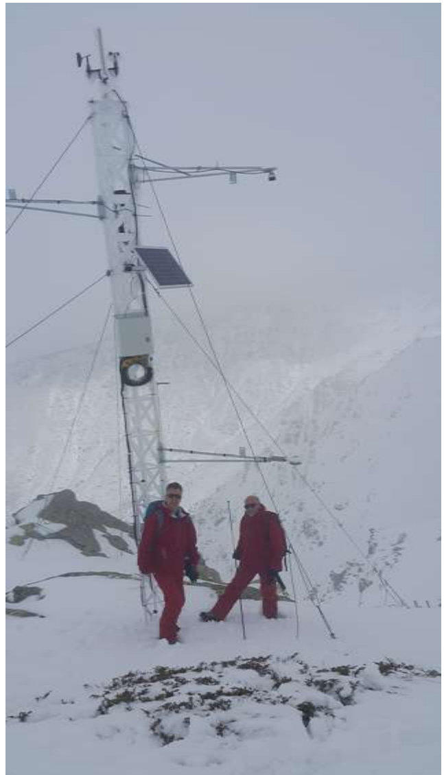
Fig 6. Automated Weather Station For Avalanche Studies on Bozdag Summit (O. Kocyigit and G. Arslan)
