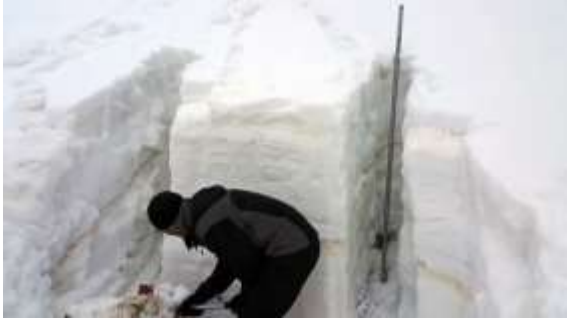
Fig 5. Snow Pit on Bozdag North Face and Simple Snow Stability Tests (Dr. E. Tekin)
