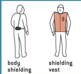
For rescue critical devices (radio, transceiver), use body shielding and / or shielding vest.
