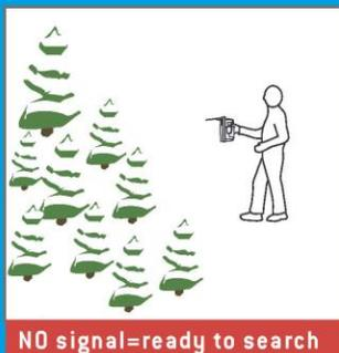
Point device to reflection-free horizon. Make signal search motion.
