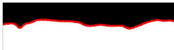
Figure 4: Method used to determine the width of the cornice. Top: original image corrected for camera movement. The red square shows the part of the cornice we analyzed. Bottom: cornice section converted to black and white and rotated. The red line shows the location of the edge of the cornice.
