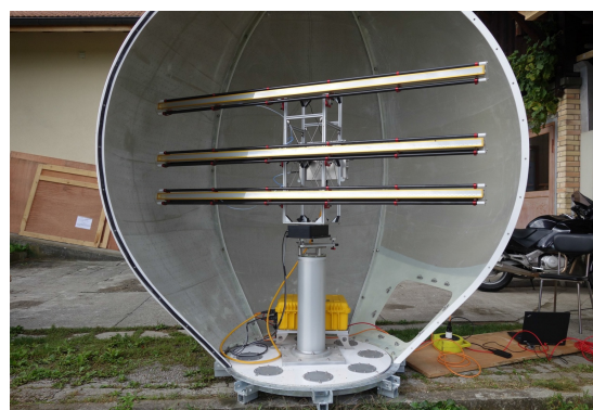
Fig. 2: Gamma Portable Radar Interferometer (GPRI) with a height of about 2.2 m and a weight of 45 kg, installed in a radome at SLF.
