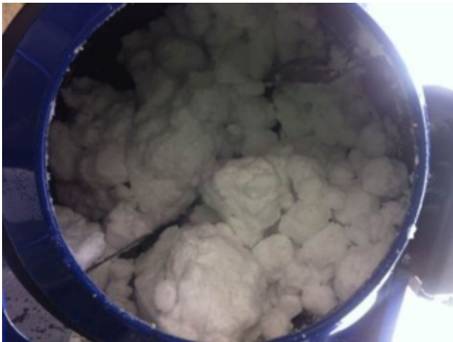
Fig. 3: Persistent-moist granules that formed inside the tumbler.
