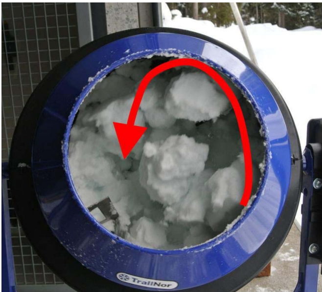
Fig. 1: Granules in motion in rotating tumbler. One (of the two) mixing blades can be seen at lower left corner.
