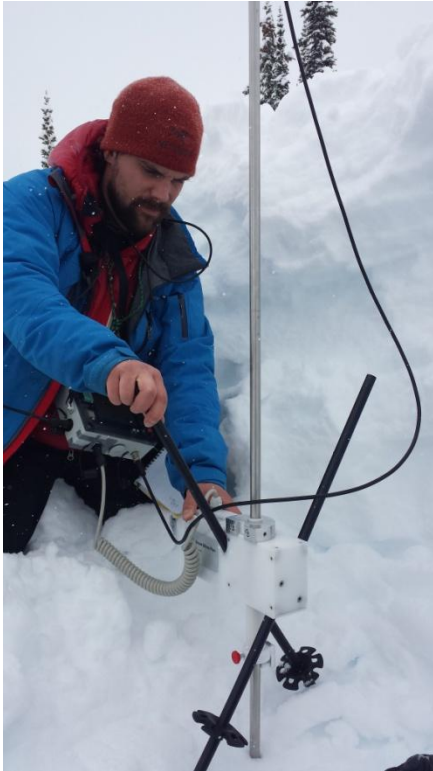
Fig. 2: The author performing a 270cm SMP profile at Mt Fidelity study plot.
