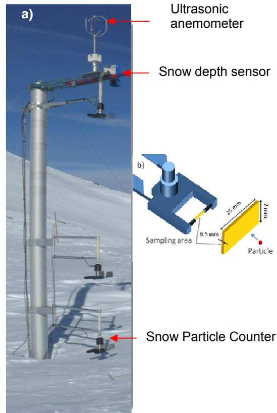
Fig. 2: a) the mast with 3 Snow Particles Counters, one snow depth sensor and an ultrasonic anemometer set up at Lac Blanc Pass
