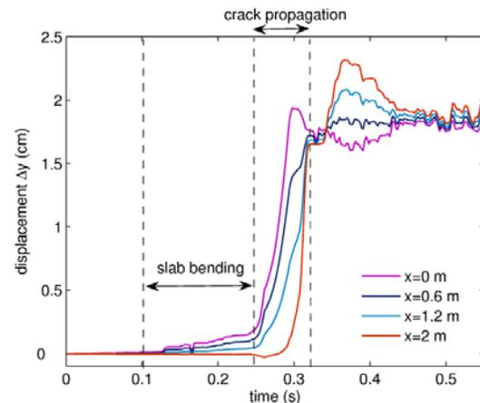
Fig. 4. Temporal evolution of the modeled vertical displacement  $\Delta y$  of the slab for a slab density  $\rho = 250 \text{ kg/m}^3$ . The different curves correspond to different horizontal positions of the slab, from the left-end ( $x = 0 \text{ m}$ ) to the right-end ( $x = 2 \text{ m}$ ).
