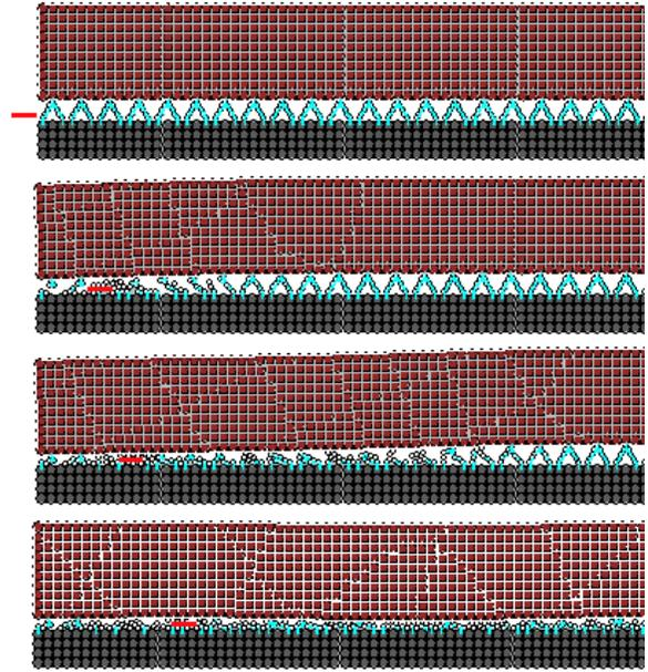
Fig. 3. Snapshots of a PST numerical experiment. (a) Initial system  $t = 0.1 \text{ s}$ , (b) onset of crack propagation  $t = 0.26 \text{ s}$ , (c) dynamic propagation  $t = 0.28 \text{ s}$ ; (d) complete failure of the WL  $t = 0.45 \text{ s}$ .
