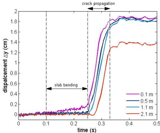
Fig. 5: Temporal evolution of the measured vertical displacement  $\Delta y$  for a slab density of  $\rho = 240 \text{ kg/m}^3$ . The different curves correspond to different horizontal positions of the slab, from the left-end ( $x = 0 \text{ m}$ ) to the right-end ( $x = 2 \text{ m}$ ).
