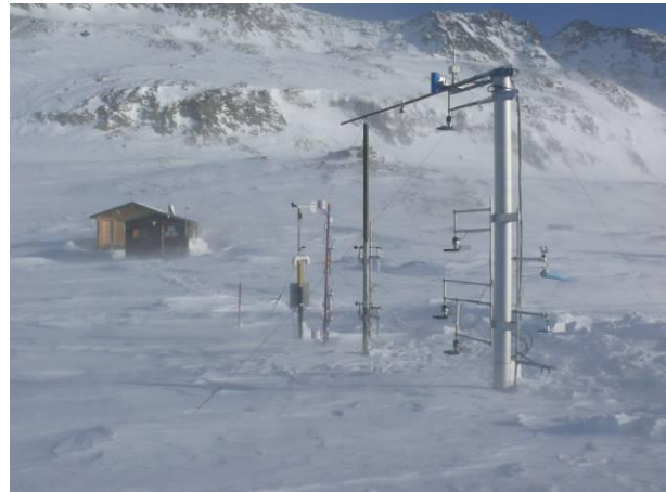
Figure 12. New configuration for winter 2012-2013 / Four Snow Particles Counters and Six anemometers
