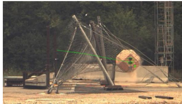
Figure 7. 1:1 field test with 500 kJ on a SPIDER Avalanche System performed at Dynamic Test Center DTC in Vauffelin, Switzerland.
