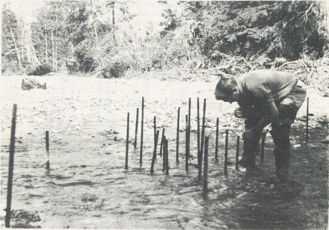
Figure 4.--Randomly placed standpipes at depths of 5, 10, 15, and 20 inches, experiment 1, Indian Creek, 1958.
