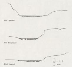
Figure 8. Representative stream channel cross sections from the 1979 hydraulic and channel geometry analysis.
