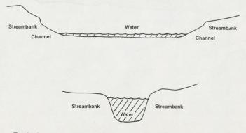
Typical stream channel cross section in the lightly and heavily grazed sites. Upper is the heavily grazed area, lower is the lightly grazed area.
