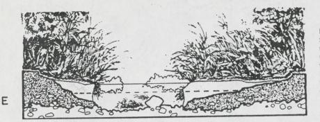
MIDSUMMER A FEW YEARS LATER: Silt bars further stabilized by turf. Channel narrowed by 40% to 50% since stage A. Only 2 feet of stream width exposed; therefore submergents less abundant. Also less volume of watercress due to shade of taller plants. Woody vegetation starting to dominate.
