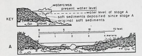
MIDSUMMER CONDITIONS UNDER HEAVY GRAZING BY LIVESTOCK: Bank vegetation and watercress grazed and trampled. Banks eroding, and stream bed mostly covered by shifting silts. Submergent plants grow poorly. Whole surface of water and stream bed exposed to sun. Greatest depth in cross-section only 9 inches (22 cm). These conditions offer trout no shelter, no place to spawn, little food, and frequently unfavorable temperatures.
