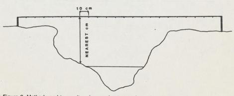
Figure 2. Method used to monitor changes in stream channel profile.
