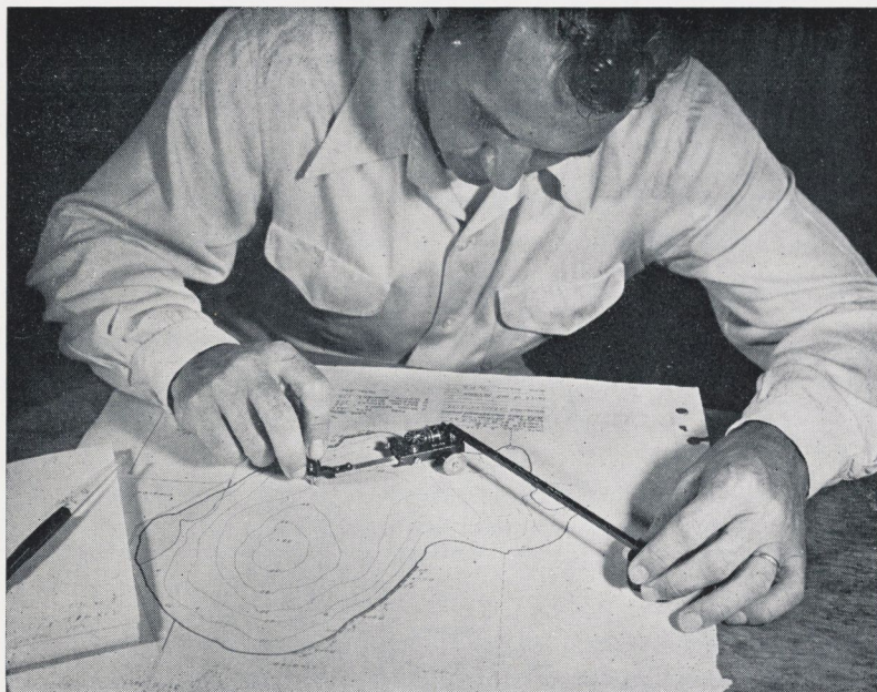
Plotting depth of lake to determine volume of water Photo by Leon Johnson, courtesy Fish Management Division, State of Wisconsin
