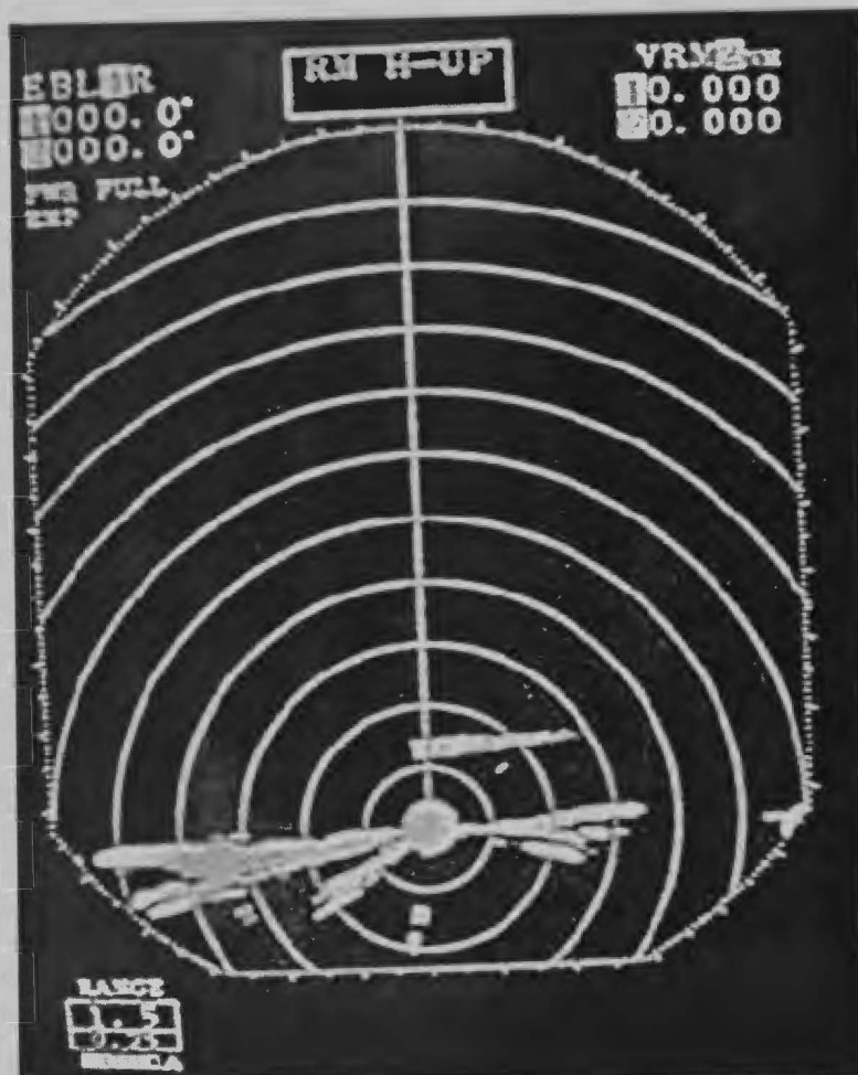
Figure 1. Screen of radar (center of concentric rings) in vertical mode displaying an event signature, probably a flock of Canada geese, moving from right (east) to left (west). Height of flock is approximately 470 m above radar. Horizontal irregular blob is ground level.
