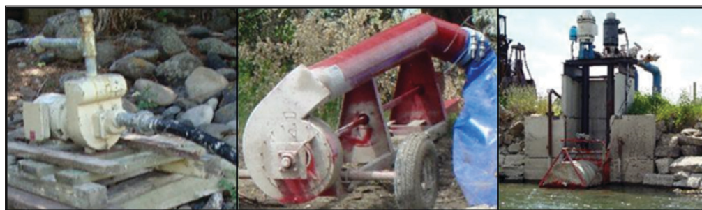
Figure 2. Examples of domestic, centrifugal, and turbine pumps.
