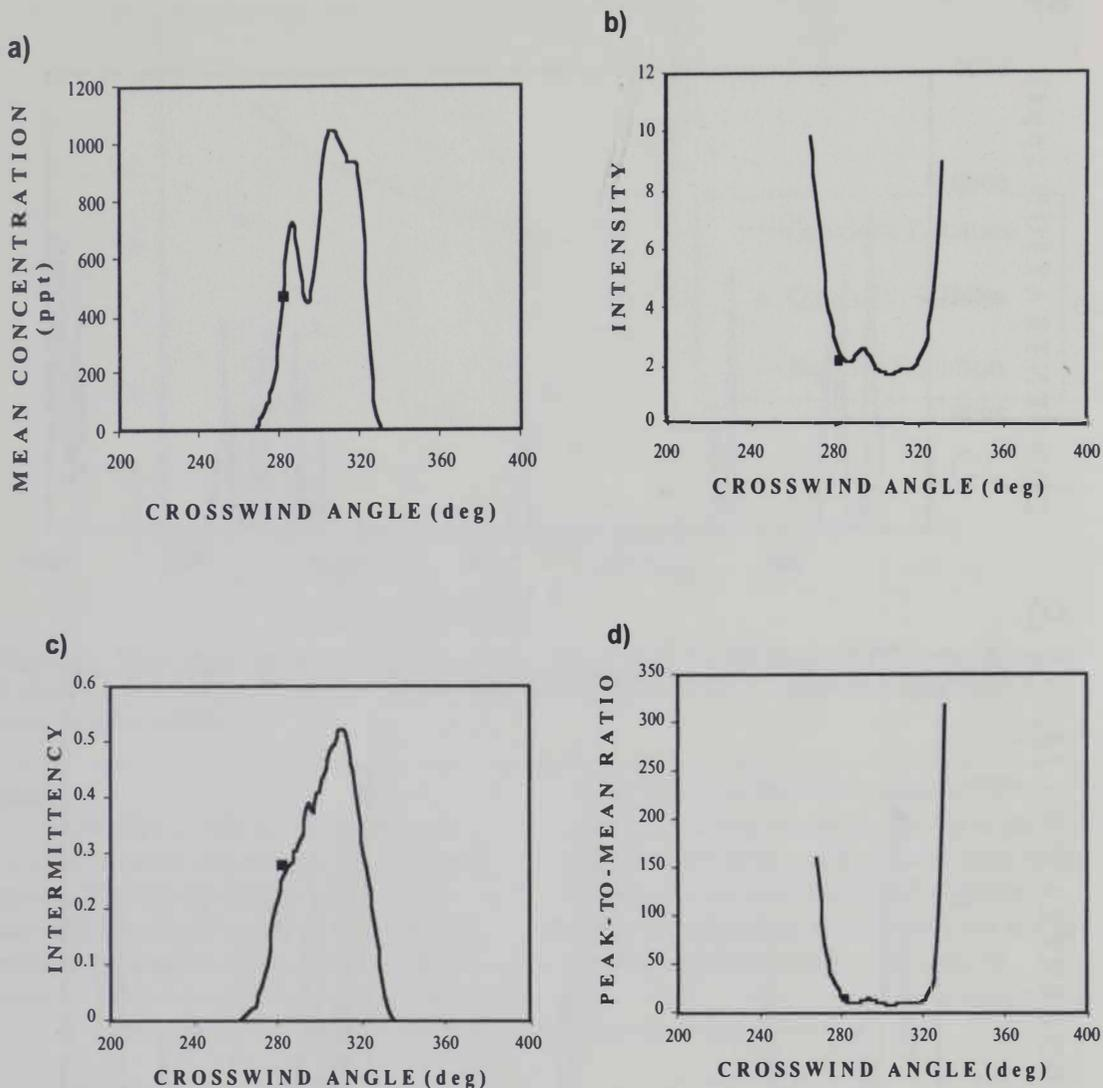
**Figure 6.** Crosswind profiles from the MIND model for test S808d, including a) mean concentration, b) intensity, c) intermittency, and d) peak-to-mean ratio. The statistic for the observed time series (shown in Figure 5a) is indicated by a "square".
