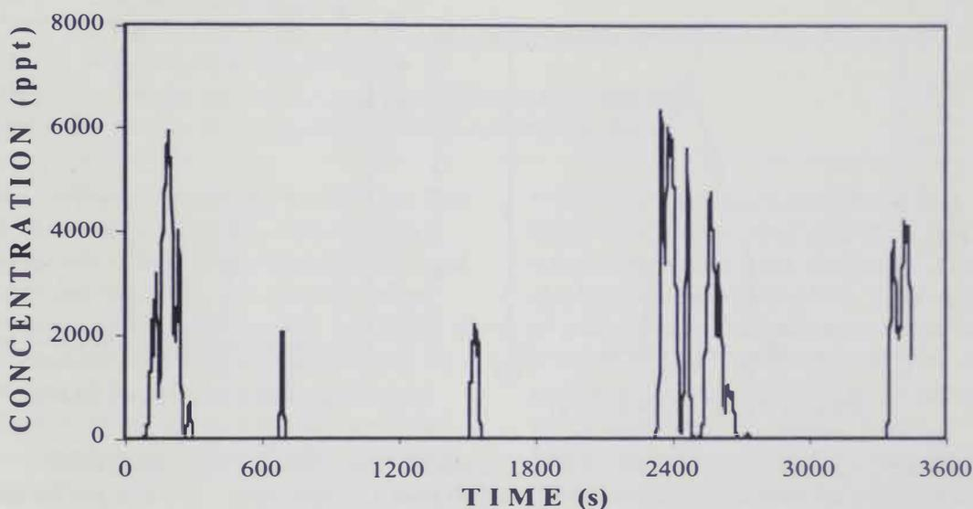
**Figure 5.** Concentration data for test S808d including a) time series of observations from the fast-response SF<sub>6</sub> analyzer at a receptor angle of 282°, b) predictions from the MIND model using Equation (8) for the diffusion coefficient. Also shown are 1:1, 1:2, and 2:1 lines-of-correspondence.
