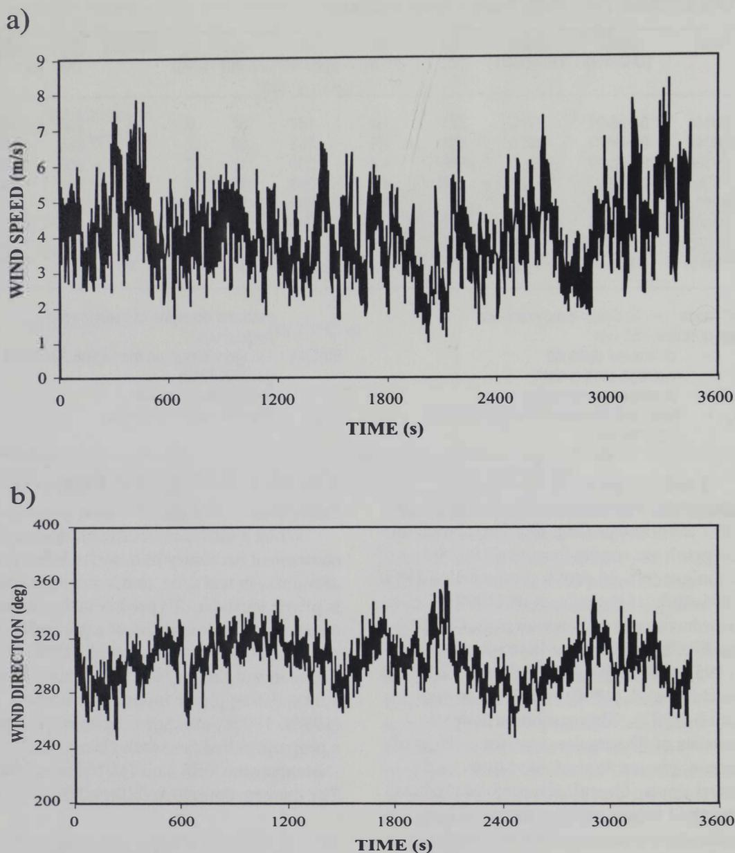
**Figure 2.** Time series of a) wind speed and b) wind direction for test S808d. Statistics include an average wind speed of  $4 \text{ ms}^{-1}$ , an average wind direction of  $303^\circ$ , and a standard deviation of wind azimuth of  $19^\circ$ .
