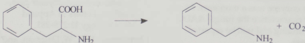
Figure 2. Decarboxylation of L-phenethylamine to yield phenethylamine, 1 .
