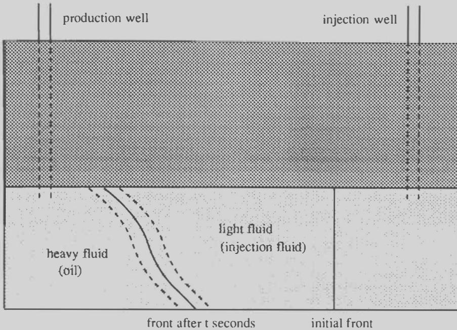
Figure 1. Motion of the front inside the reservoir
