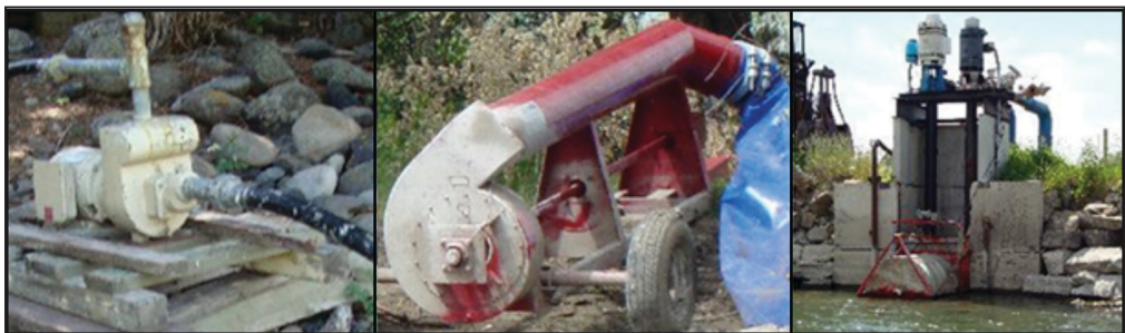
Figure 2. Examples of domestic, centrifugal, and turbine pumps.
