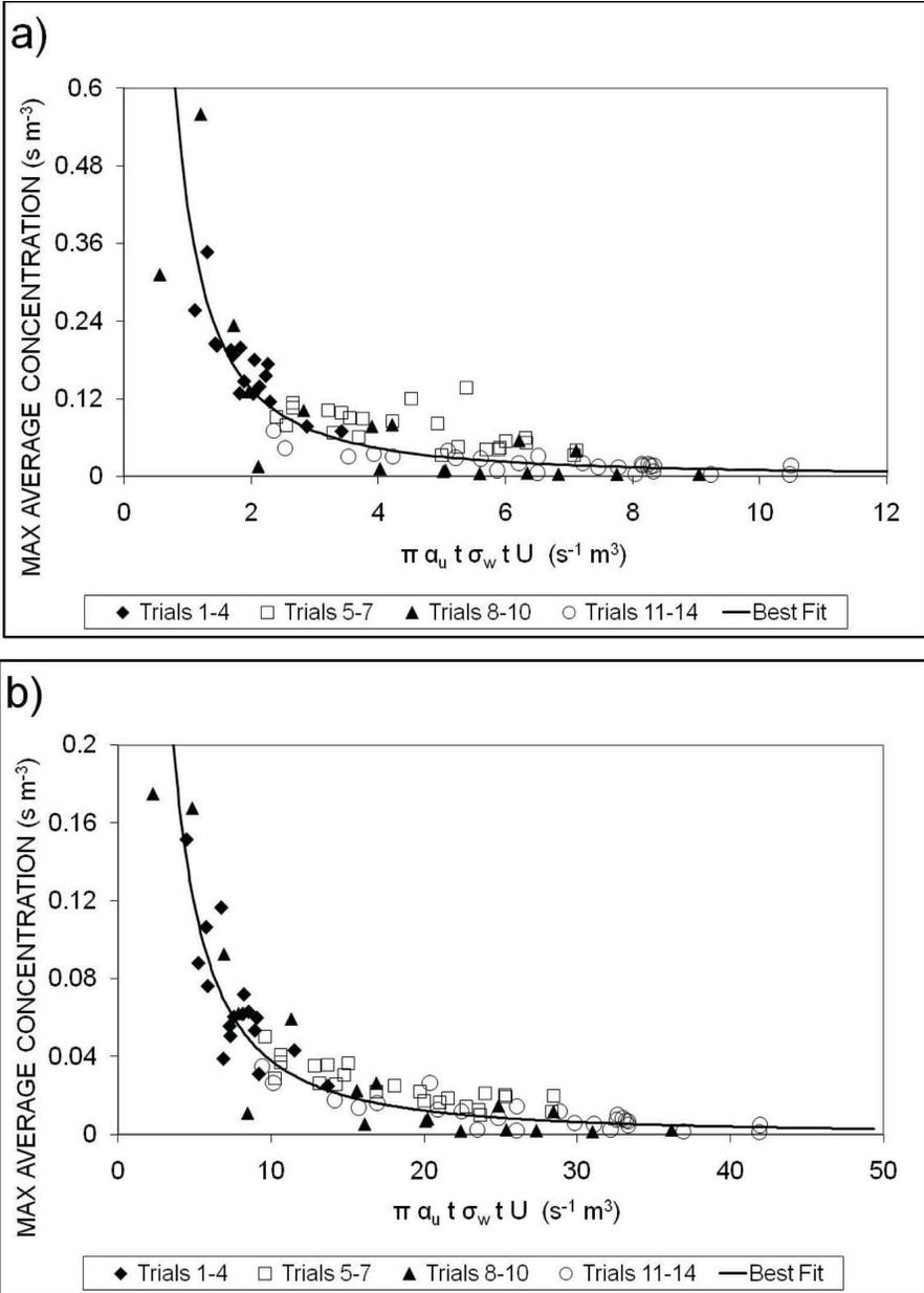
Figure 4. Maximum average concentration versus  $\pi \sigma_u t \sigma_w t U$  for the: a) 5-m arc, and b) 10-m arc for all tests.
