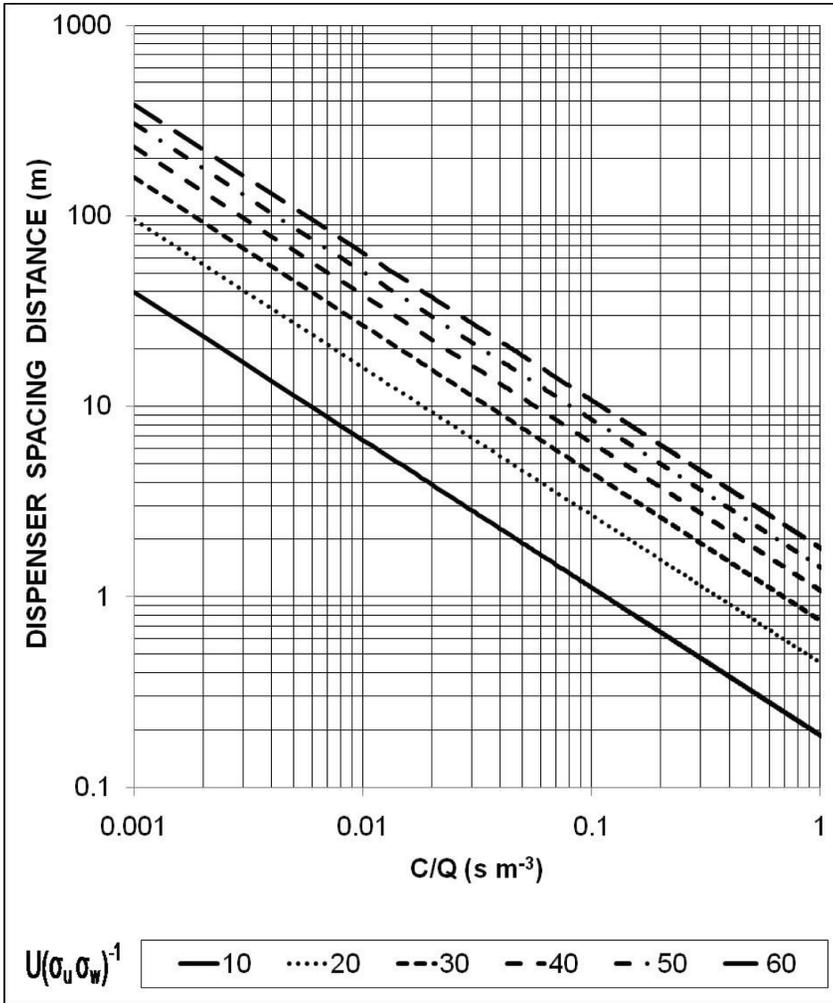
Figure 6. Example field chart of dispenser spacing distance versus maximum average concentration for  $U(\sigma_u \sigma_w)^{-1}$  ranging between 10 and 60. [Units on  $U(\sigma_u \sigma_w)^{-1}$  are  $s\ m^{-1}$ .]
