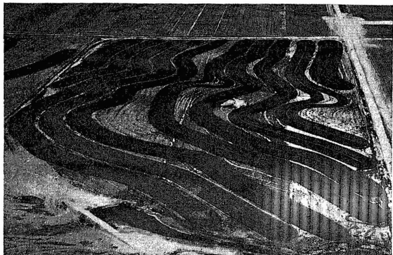
Fig. 18. Contour strip farming in the Soil Conservation Service demonstration area in Roosevelt County. This system guards against both wind and water erosion. (Photo by 41st Division Aviation, Washington National Guard.)
