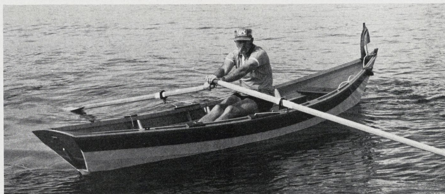
Versatile Dory. Adapted from fixed-seat rowing, the Atlantic Skiff is meant for and attuned to open-sea handling. She can also be rigged as a sailboat.
