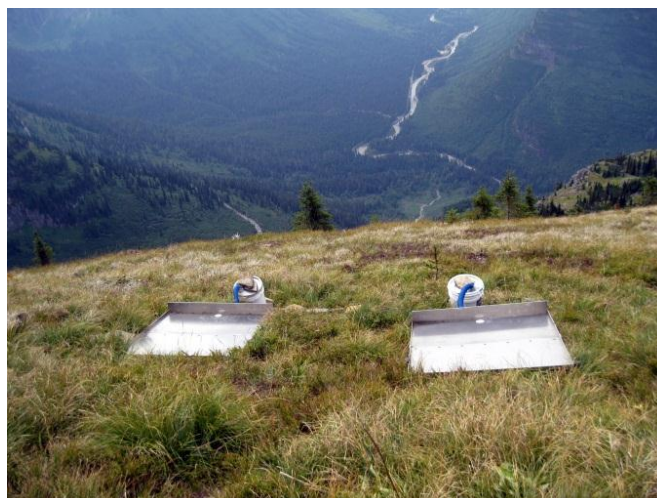
Figure 2: Two lysimeters installed on a 30 degree slope adjacent to GWWX to record local water flow through the snowpack. This image was taken looking downhill.
