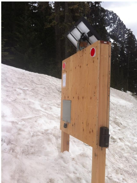
Figure 4. Rear of the Beacon Check Station. The solar panel is mounted to the top of the structure and the beam sensor to the side post.
