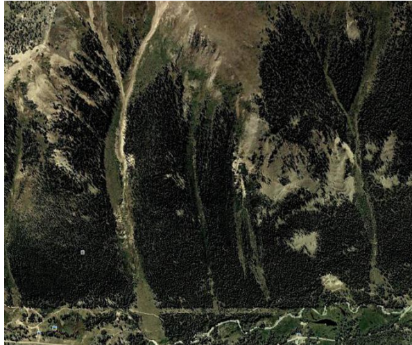
Figure 1: Before and after images of the High Voltage path: Before the 2011 event, the lower track and runout had grown in with trees, and the area of new damage to the west of the path was densely forested. The High Voltage path now clearly intersects the power line and Peru Creek in the runout zone, and the track is almost as wide as the adjacent Corkscrew path. Images were collected June 30, 2008 (above), and Sept 23, 2011 (below), Google Earth 2012.
