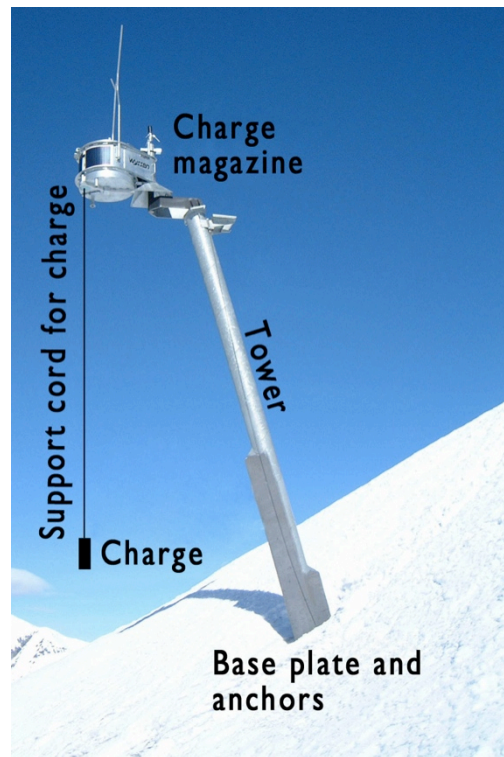
Figure 2: Overview over the Wyssen avalanche tower with the main components highlighted.
