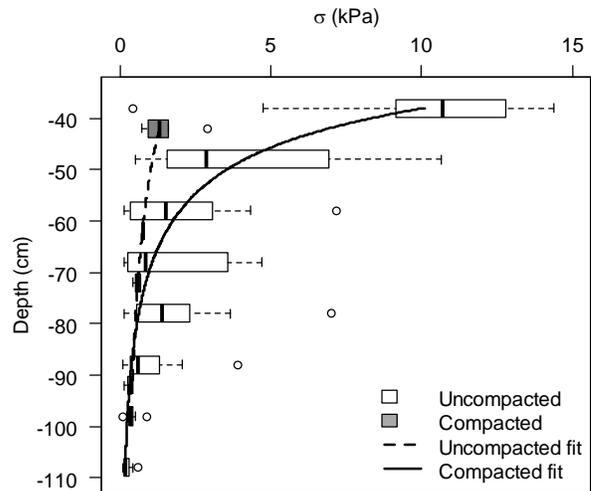
Figure 7: Distribution of stress per depth for snowmobiles. Grey box plots correspond to data collected where the surface of the snowpack was artificially compacted and supported the LDL. White box plots correspond to data collected where the surface of the snowpack was undisturbed, soft and allowed penetration of the LDL (uncompacted). Lines indicate the fitted models. Boxes, whiskers and open circles as in Figure 2.
