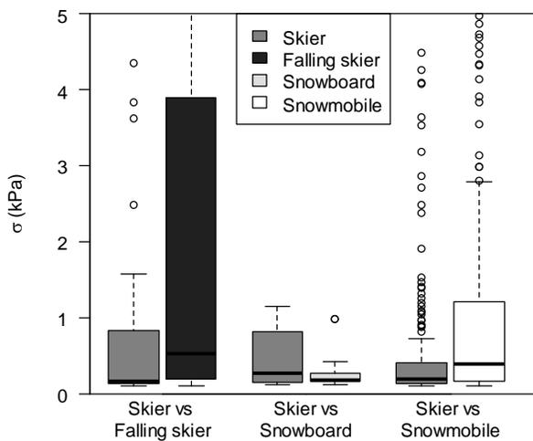
Figure 6: Stress for varying triggers compared to skiers. Boxes, whiskers and open circles as in Figure 2.
