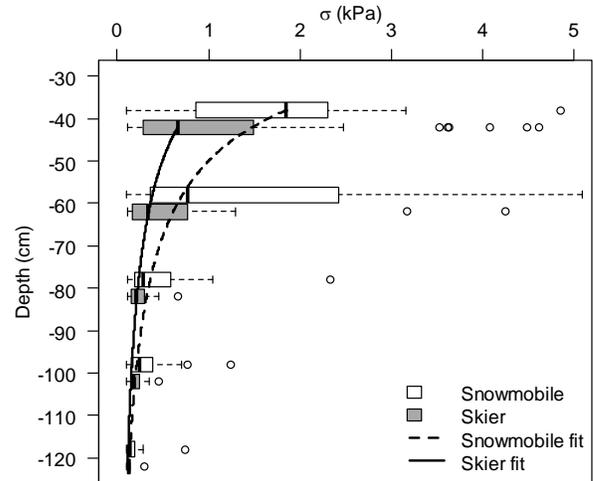
Figure 2: Box plots of stress by absolute depth class for snowmobiles (white) and skiers (grey). Lines indicate the fitted model for snowmobiles (dashed) and skiers (solid). Boxes span the interquartile range. Whiskers extend to 1.5 times the interquartile range. Open circles indicate outliers.
