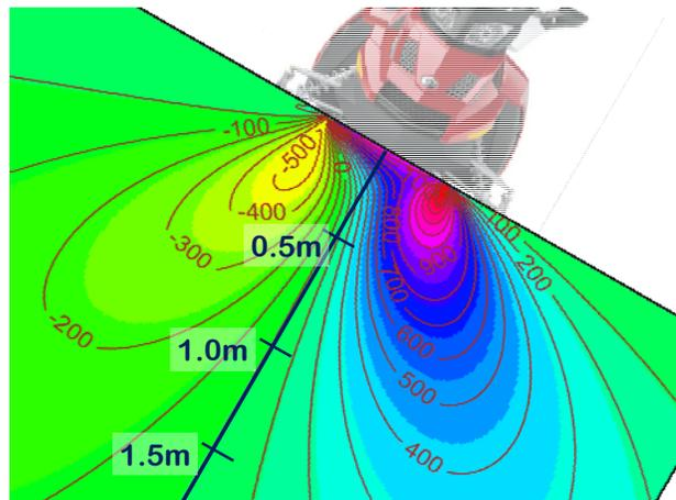
Figure 5: Static shear stress below a snowmobile (Calculations based on Das 1983)
