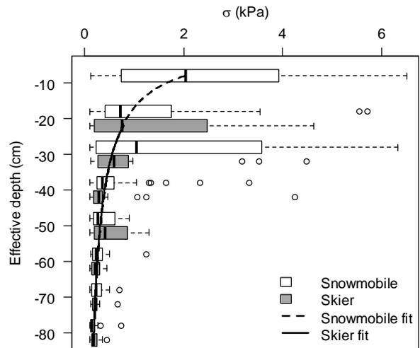
Figure 3: Box plots of measured stress per effective depth (penetration depth subtracted from depth) for snowmobiles (white) and skiers (grey). Lines indicate the fitted model for snowmobiles (solid) and skiers (dashed). Note, the fitted lines overlap each other. Boxes, whiskers and open circles as in Figure 2.
