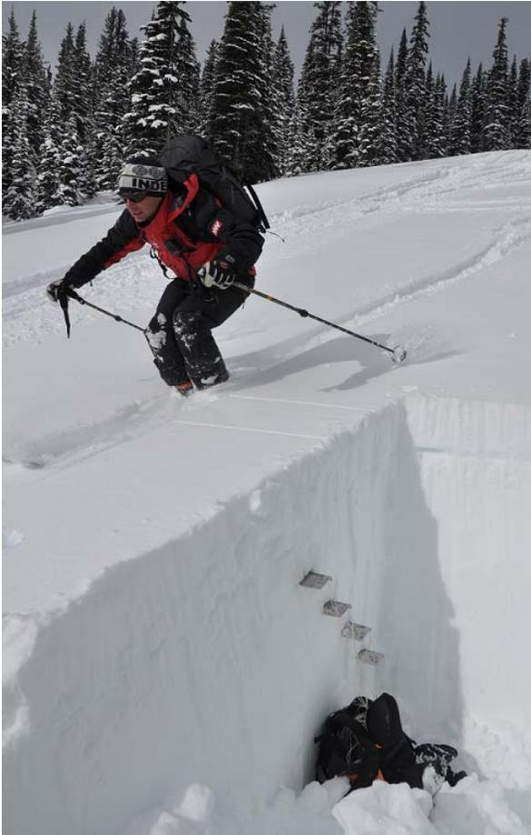
Figure 1: Skier performing an experiment loading the snow surface above the buried sensors.
