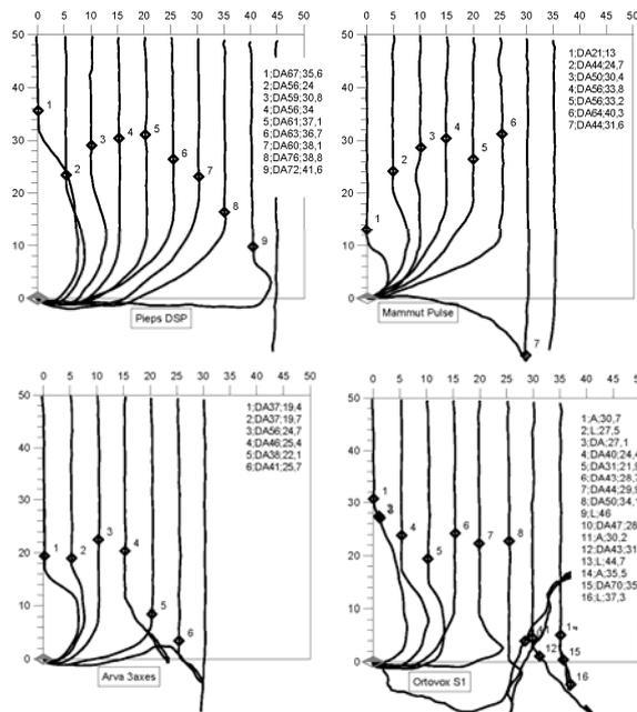
Fig 4. Trajectories of four different 3-antenna beacons in bed coupling position. The numbered points indicate the first signal and are discussed in the text. The useful range of the beacons, clockwise from the top left are 40 m, 30 m, 25 m, and 25 m.
