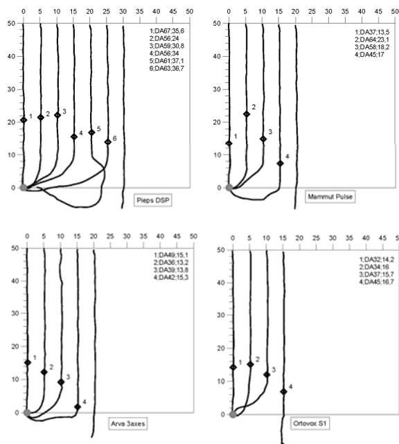
Fig 5. Trajectories of four different 3-antenna beacons with a vertical transmitter antenna. The numbered points indicate the first signal and are discussed in the text. The useful range of the beacons, clockwise from then top left are 25 m, 15 m, 15 m, and 10 m.
