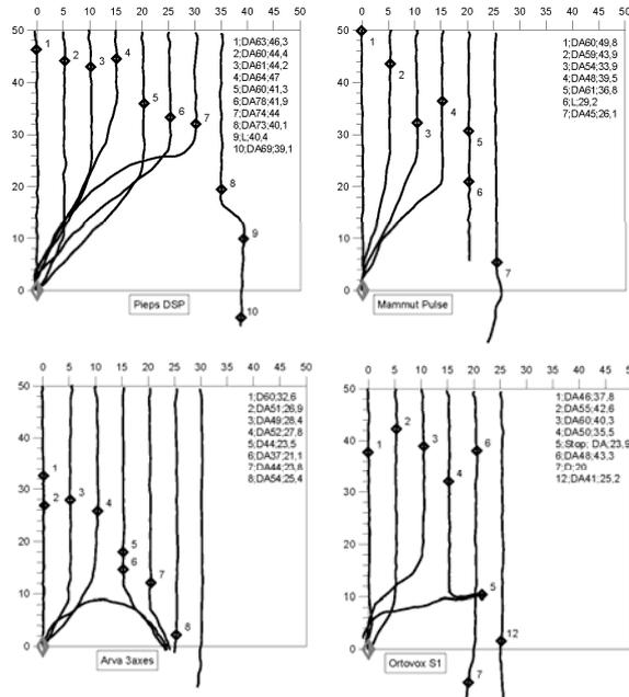
Fig 3. Trajectories of four different 3-antenna beacons in good coupling position. The numbered points indicate the first signal and are discussed in the text. The useful range of the beacons, clockwise from the top left are 30 m, 15 m, 20 m, and 15 m.
