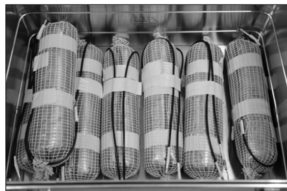
Figure 6. Prepared charges for helicopter blasting.
