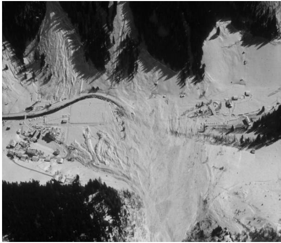
Figure 6. Clear distinction of powder snow and dense snow deposition
