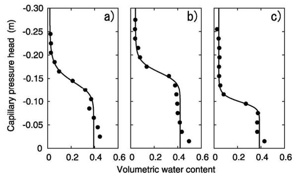
Figure 2 Water retention curve for drying in a) sample  $S_S$ , b) sample  $S_M$ , and c) sample  $S_L$ . Marks indicate the measured water retention data, Solid lines indicate WRC fitted with van Genuchten's model.
