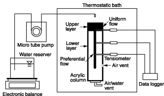
Figure 1 Schematic diagram of the experiment for measuring the water-entry values.
