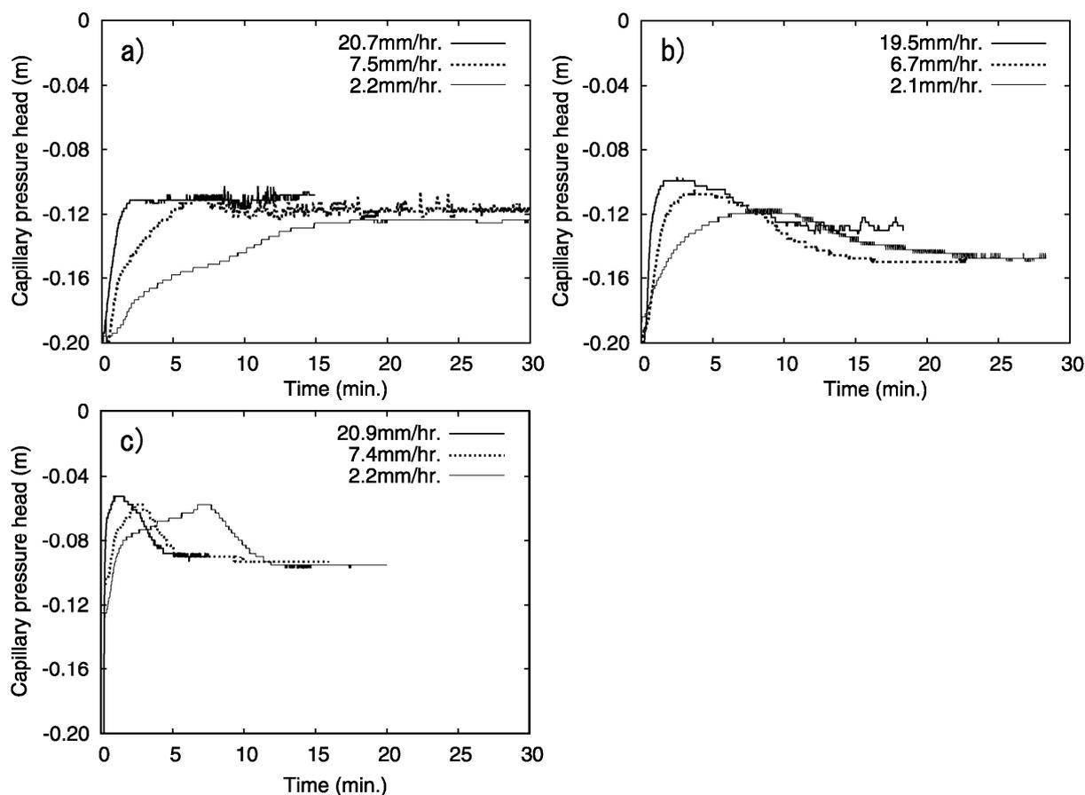
Figure 3 behaviour of capillary pressure head measured in the samples of a)  $S_S$ , b)  $S_M$ , and c)  $S_L$ .
