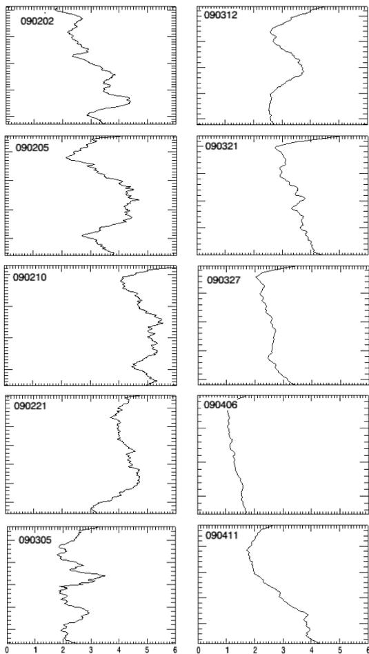
Figure 4: Evolution of the horizontally averaged vertical SSA for crust CR090127. Order of evolution is top to bottom, left column then right at 1 week intervals.
