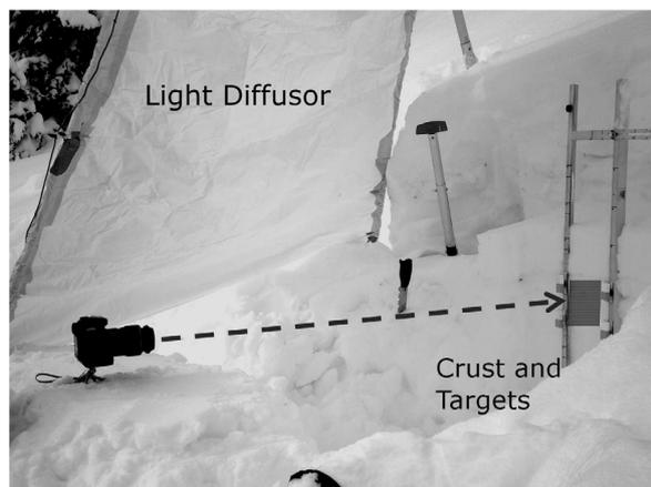
Figure 1: *Equipment and configuration used for near infrared photography.*
