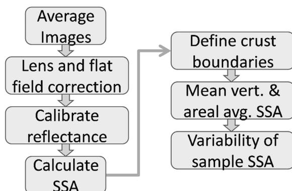
Figure 2: *Post-processing of near infrared crust images.*
